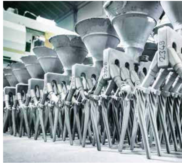
Cast blanks for hip prosthesis stems at VACUCAST®
